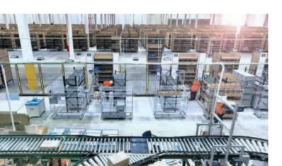
An automated conveyor system ensures on-time processing and fast delivery times to establish the best customer experience for adidas, a global leader in the sporting goods industry and DB Schenker's leading customer in this site. In order to optimize the volume of parcels and utilization of transport vehicles, packaging is adjusted to the exact size of the product that is shipped through an automated solution. This results in reduced CO2 emissions throughout distribution.
